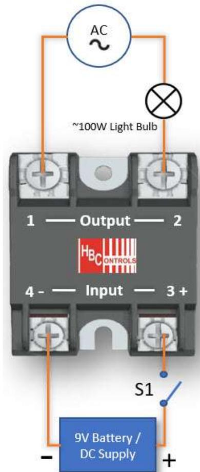
**Fig. 1 – DC Input / AC Output Solid State Relay Test Setup**
