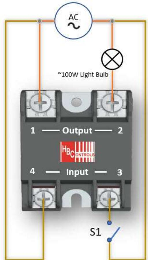
**Fig. 2 – AC Input / AC Output Solid State Relay Test Setup**
