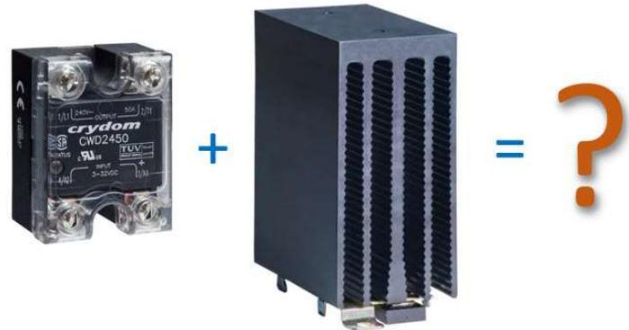
A decent, SCR-based solid-state relay will dissipate power at a rate of about 1 Watt per ampere of load current. Once the load current exceeds five to seven amps, an external heat sink is required to ensure that the relay doesn't overheat. Therefore, for example, a 50-amp rated SSR is *only* rated for 50 amps when mounted to a heat sink that can adequately dissipate 50 Watts of power. Failure to provide an adequate heat sink will result in excessive temperatures and, ultimately, relay failure.
